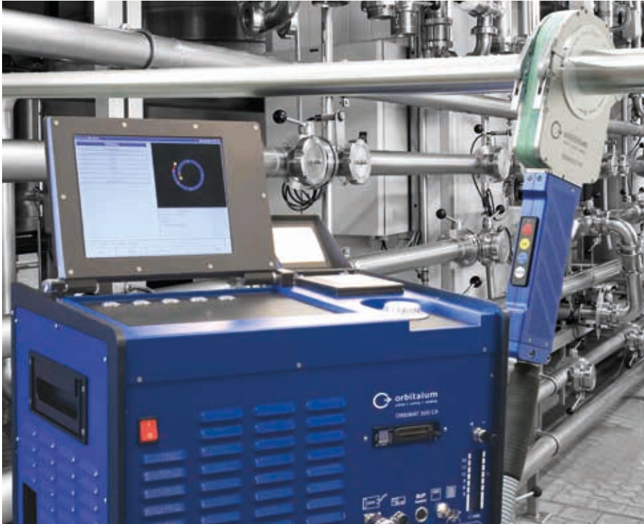
10.5" swivel monitor and system printer integrated
